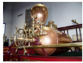
A 40 gallon chemical tank is onboard and the large brass balloon shaped dome is an accumulator tank to absorb shock when the hoses are turned on or off.
