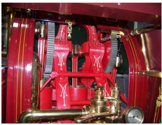
Jumbo carries a 3 piston positive displacement pump that delivered 750 gallons per minute.
