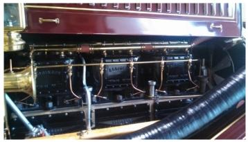
Jumbo is powered by a 6 cylinder gasoline engine, built by Buffalo Marine, with a displacement of 1245 cubic inches that produced 150 horsepower. The cylinders are cast in pairs. These engines were used in early tugboats.
