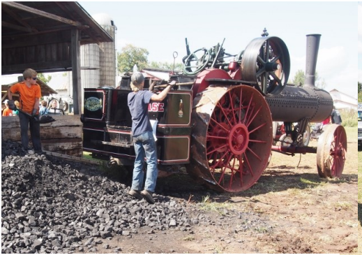
This was the fueling station where coal was being shoveled into a hopper that would later be stoked into the boiler to generate steam. Pumping gasoline into later tractors was a major breakthrough.
