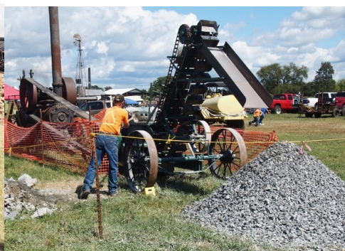
My favorite (and the loudest) operation was this steam powered rock crusher turning big ones into little ones.
